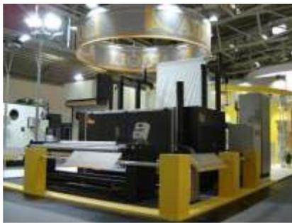
The machine realized for the project "Metadistretti per l'eccellenza Lombarda", with "ARIOLI s.p.a.", textile machinery enterprise, as leader company, together with the research institutes "Stazione Sperimentale per la Seta" and "Plasma Prometeo" of "Università degli Studi – Milano-Bicocca" is based on DBD-type discharges, it operates under atmospheric pressure with air or inert gases and several gas mixtures, it produces plasma between two or more electrodes in which the fabric run.
