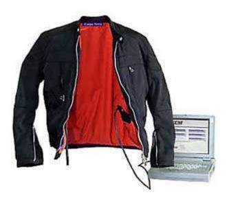
Inside the jacket lining is a computerized microprocessor with hard disk (no bigger than a packet of cigarettes) which controls the body temperature over a series of electric heating pads.
